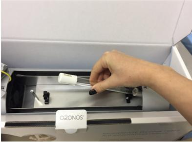
5. Now lift the lamp first on the left, then on the right side out of the bracket and carefully pull the lamp out of the plug.
