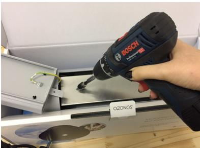
3. Put the outer case aside and unscrew the screw of the inner case.
