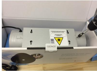
2. Unscrew the two screws with a Torx I0 screwdriver.
