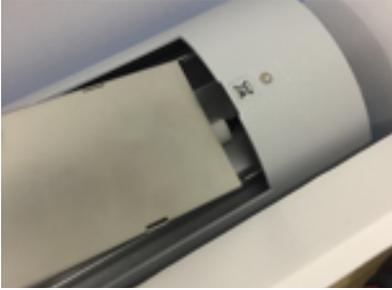
9. Reassemble the inner case. Start by inserting the inner case as far to the right as possible and then slide it to the left. Now retighten the screw to fix the inner case.
