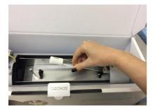
5. Now lift the lamp first on the left, then on the right side out of the bracket and carefully pull the lamp out of the plug.
