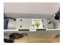
2. Unscrew the two screws with a Torx IO screwdriver.
